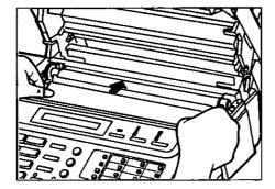
Insert the leading edge of recording paper between the upper and the lower guide plates.
