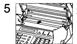
Then insert its leading edge between upper and lower guide plate and pull the paper a few centimeters (one or two inches) out of the unit.
