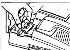
Insert the microcassette tape into the compartment with the full reel to the left.
