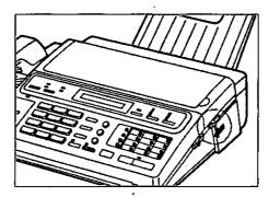
Slide the **BACK LID OPEN** lever forward to open the paper compartment cover.
