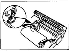
Insert the left projection of the paper roll holder into the left groove on the unit then the right projection into the right groove, while pushing the paper roll to the left.
